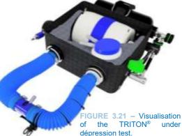
Observe the counterlungs and ringed hoses (the reabreather flexible parts) and watch for a possible change due to the filling of the loop. This test must last at least one minute.
